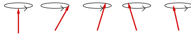
Figure 6.6: FM spin wave: all spins are originally aligned along the z -axis and subsequently tilted by the presence of a magnon. Precession frequency is determined by the \omega vs. \vec{k} dispersion relation. In this figure, the phase difference is \approx \frac{2\pi}{5} .
